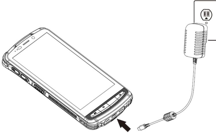
**Note:** Low battery may result in a malfunction of the terminal. Before your first use, charge the battery for at least 6 hours.
