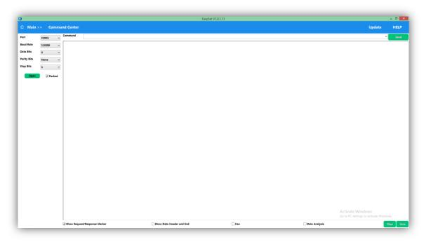
To send one (e.g. 128ENA1;) or more serial command(s) (e.g. 128ENA1;CID12841;) to a device, select the COM port connected to that device, input the command(s) in the Command field and then click on "Send".
