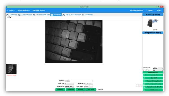
To view the real-time image/decode image stored on the connected device, select Real Time Image/Decode Image from the Image Type dropdown list and the desired image ratio, and then click on "Load Image".
