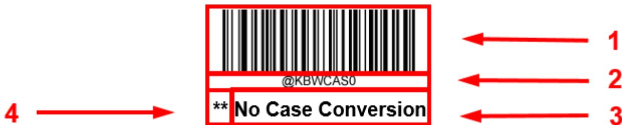
The figure above is an example that shows you the programming barcode and command for the Enter Setup function:
