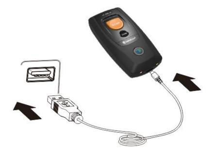
Note: Low battery may result in failure or misoperation of the scanner. Before your first use, charge the battery for 3-4 hours. Make sure the scanner is full charged before the operation
