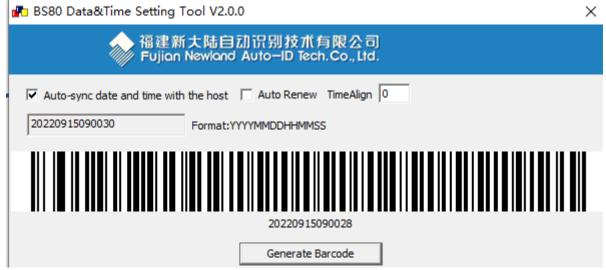
Step 3: Scan the barcode generated to set the date and time on the scanner.
